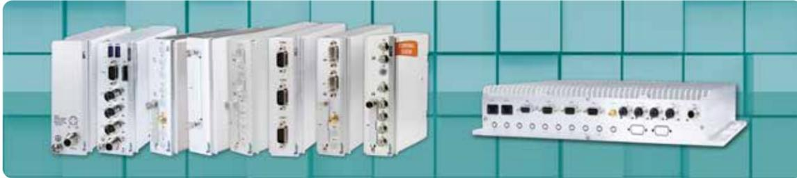
duagon's box PCs are a selection of individual prefabricated components that can combine various functions as required to create computing platforms for a range of rail onboard, wayside and industrial IoT applications. The modules are combined in flexible built-to-order configurations that can be conveniently mounted on a space-saving standard DIN-rail, wall/flat surface and 19" mounting.
